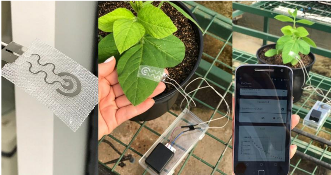
Figure 10. Folial sensor for water loss detection. Source: Um Só Planeta
