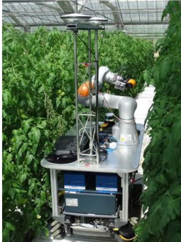
Figure 17. Green Patrol automatic dispenser for pest control. Source: SmartProtect
