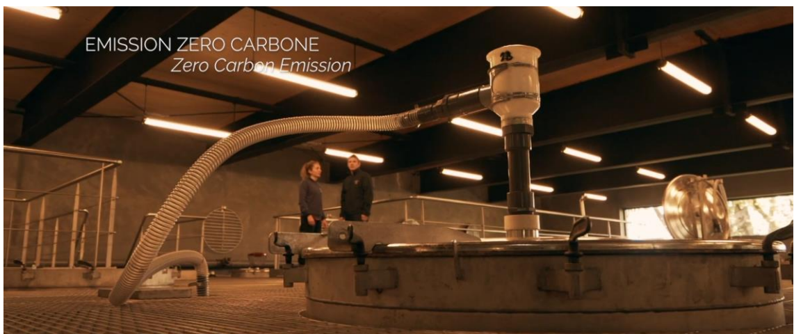
Figure 12. CO2 collector for fermentation processes. Source: Château Smith Haut Lafitte
